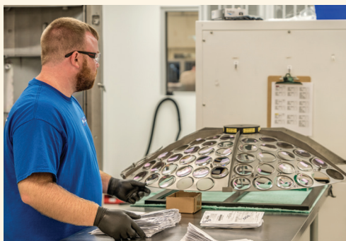
A technician inspects lenses after applying anti-reflective coating at the new VSPOne Sacramento lab.
