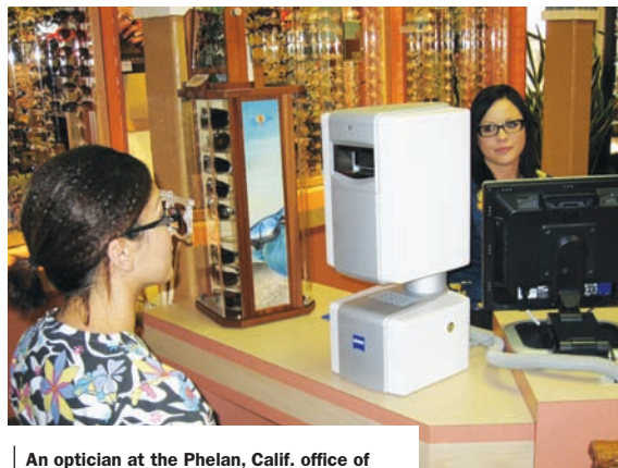
An optician at the Phelan, Calif. office of Bryan Vanesian, OD (r) uses the Zeiss iTerminal to measure a patient for Zeiss lenses.
